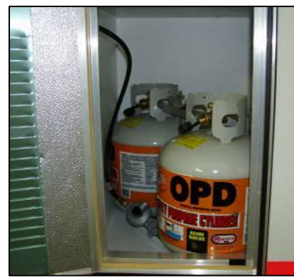
LPG System for easy bottle exchange
