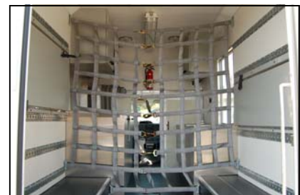
Cargo Net Installed
